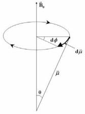
The interaction of the proton's spin with the magnetic field produces the torques, causing it to precess about the main magnetic field
