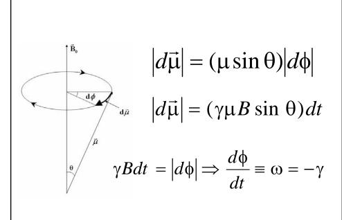
The Larmor frequency is a constant for a given static magnetic field. The magnetization vector in a volume V is defined as
